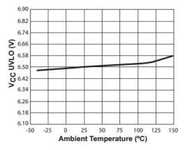
Figure 6.1 VCC UVLO vs. Temperature
