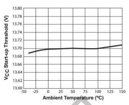
Figure 6.2 Start-Up Threshold vs. Temperature
