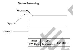
Figure 7.1: Start-up Sequencing Diagram
