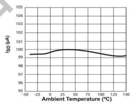
Figure 6.6 I<sub>SD</sub> vs. Temperature
