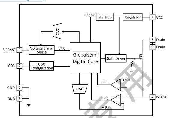
Figure 3.1 G5137PT Functional Block Diagram
