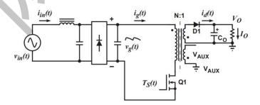
Figure 7.2: Simplified Flyback Converter
