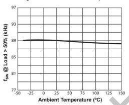
Figure 6.3 Switching Frequency vs. Temperature
