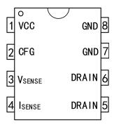
Figure 2.1: G5137PT Series (8 Lead DIP8 Package)
