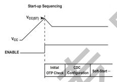
Figure 7.1: Start-up Sequencing Diagram
