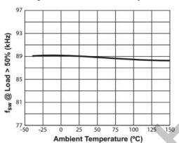
Figure 6.3 Switching Frequency vs. Temperature
