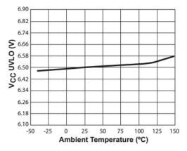
Figure 6.1 VCC UVLO vs. Temperature
