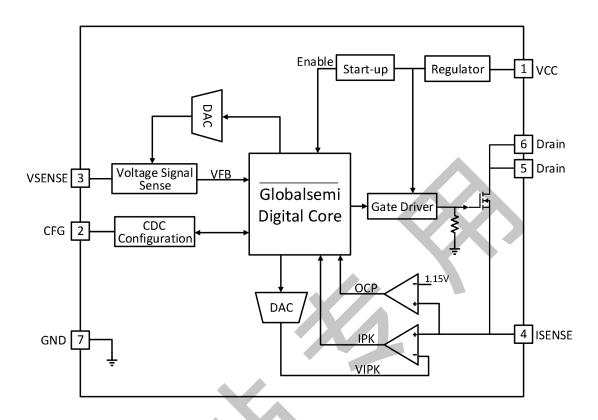
Figure 3.1 G5237FT Functional Block Diagram
