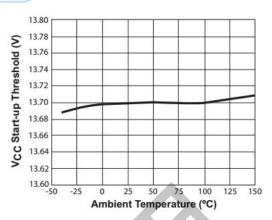
Figure 6.2 Start-Up Threshold vs. Temperature
