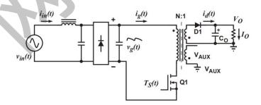
Figure 7.2: Simplified Flyback Converter
